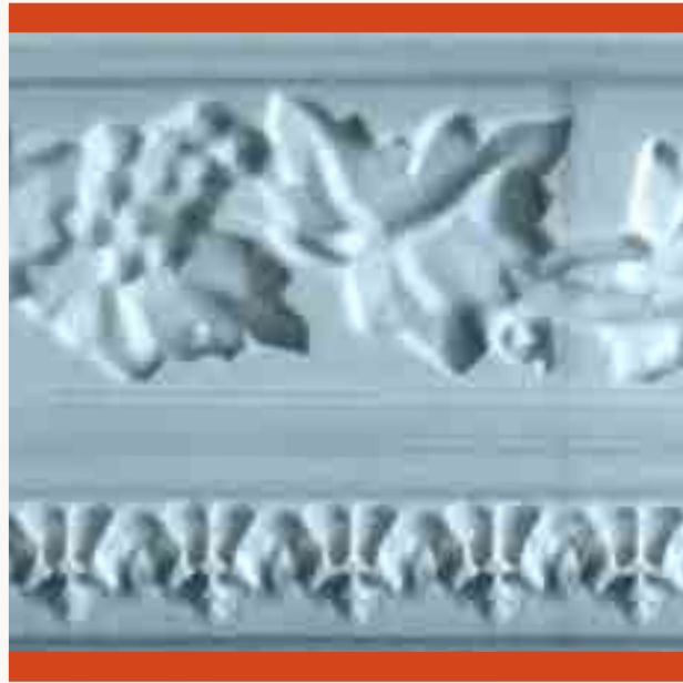
The silicone mold of the elements with the bulls' heads, obtained by the model printed in gypsum powder
